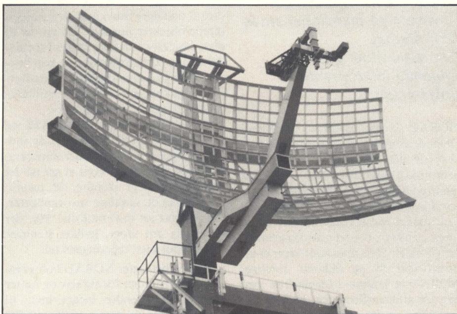
Langdistanceradar af typen ARSR-3 (Air Route Surveillance Radar) bygget af Westinghouse for Federal Aviation Administration (FAA).
